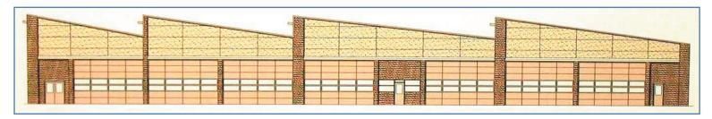
The sawtooth roof design, with high south-facing windows, provides daylighting throughout the building.
